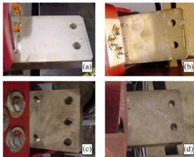
Fig. 1. Tarnished silver plating on copper bus after various periods of storage at manufacturing facility: (a) 1 month, (b) 10 months, (c) 30 months, and (d) 5 years.
