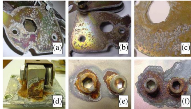
Fig. 7. Corrosion spots on steel parts from the breaker: (a)–(c) white deposit and pits on the surfaces of the plates of laminated arms; (d)–(f) white deposit and brown corrosion products on the mounting plates and bolts (“red rust”).
