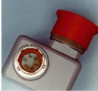
Figure 1.0 – Corroded F-16 MFSOV Electrical Connector
