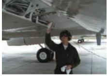
AM1 Brian Keppers of VP-30 lubricates jackscrews and flap tracks on a P-3 aircraft.
