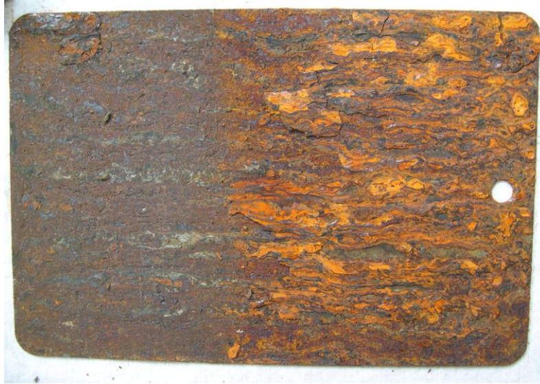
Panel 1 – No coating
