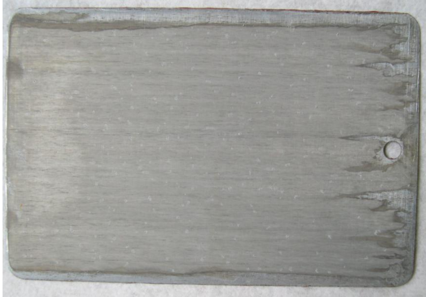
Panel 1 – No coating
