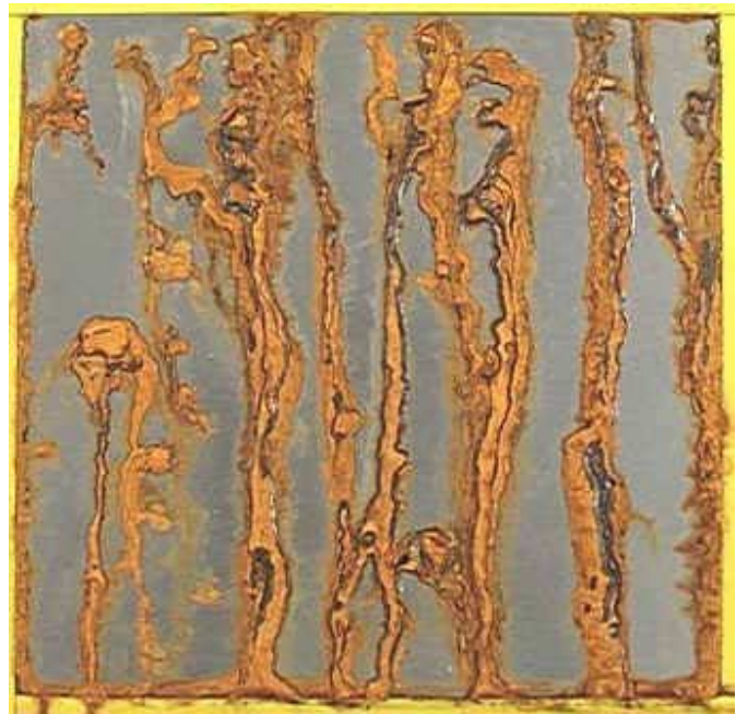
Figure 3. MIL-C-81309 Type II Treated AISI 1010 Steel Coupon Following ASTM B 117 Salt Fog Corrosion Testing (7 day).
