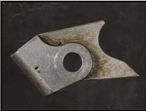
Figure 7c. CRES pawl showing pin hole.
