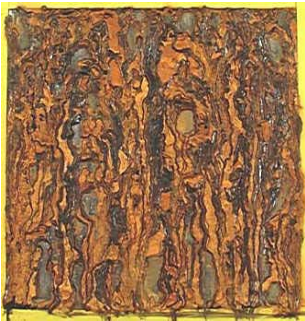
Figure 2. VV-L-800 Treated AISI 1010 Steel Coupon Following ASTM B117 Salt Fog Corrosion Testing (7 day).
