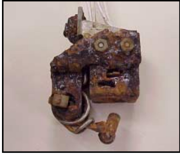
Figure 6b. Control - Electrical failure at 100 hours
