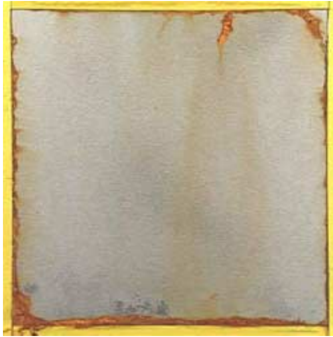
Figure 4. MIL-L-87177A Treated AISI 1010 Steel Coupon Following ASTM B 117 Salt Fog Corrosion Testing (7 day).
