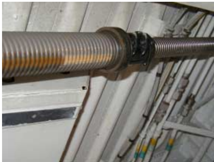
Figure 1. P-3 Jackscrew soon after water contact.
